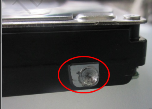
(6) Broken(Missing) Pin Guide
