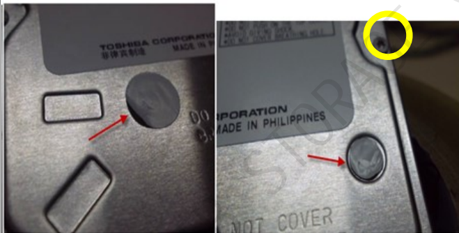
(9) Sticker on top screw slight deformed
