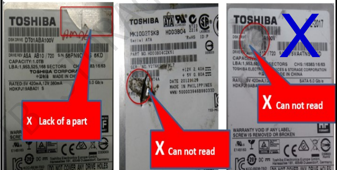
(12) Partially broken drive label (Label contents can NOT be readable)
