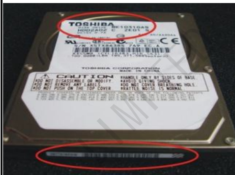
(16) Mismatch of Serial No. and Module No.
