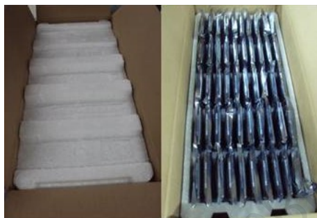
Properly packed HDDs with ESD bag, separator, inner cover & carton.
