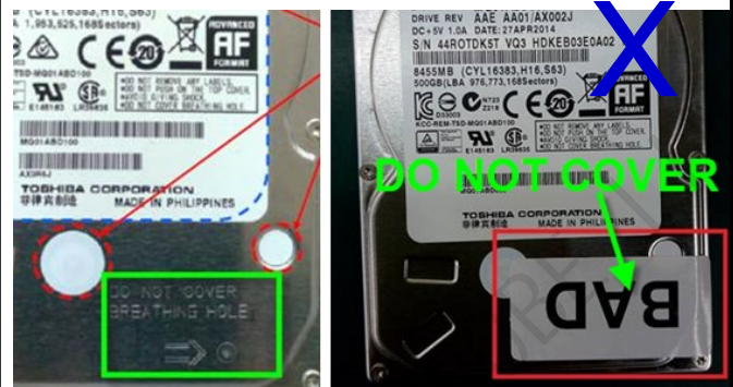
(12) Partially broken drive label (Label contents can NOT be readable)
