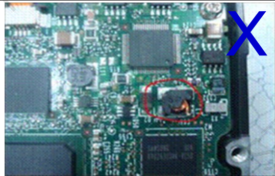
(2) PCB damage (hardware damage)
