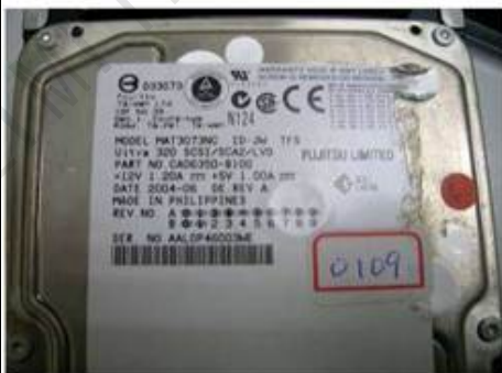
(11) Partially broken drive label (Label contents can be readable)
