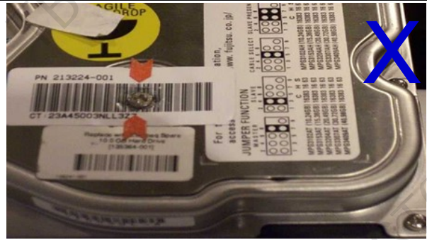
(6) Label on top screw broken
