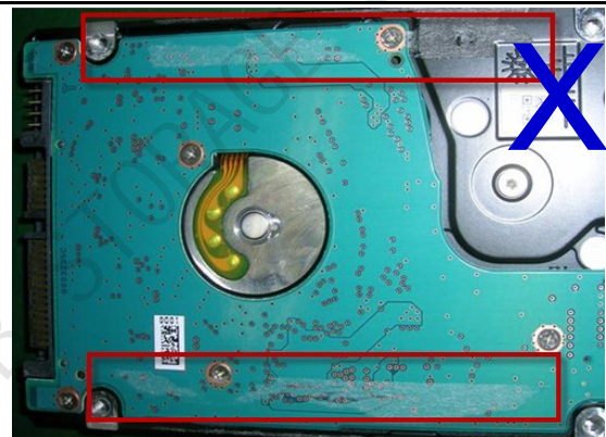
(16) Adhesion glue on PCB
