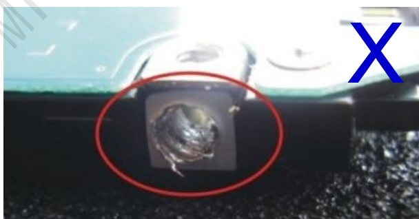
(1) Damaged screw hole
